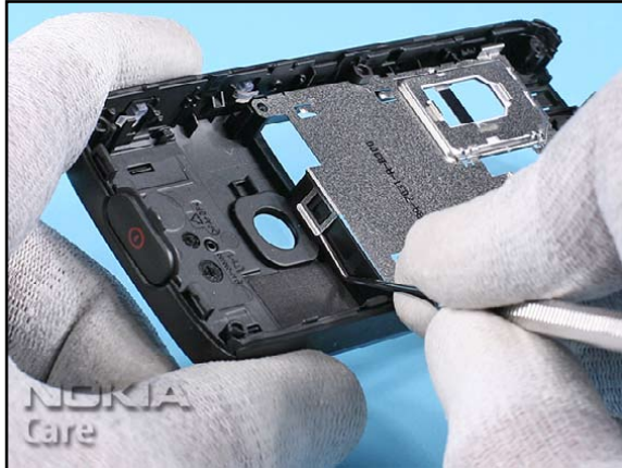
26. ...and unlock the LABEL COVER ASSY beginning at the shown side.
