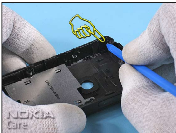
32. Release the clips of the DECO TRIM LEFT.
