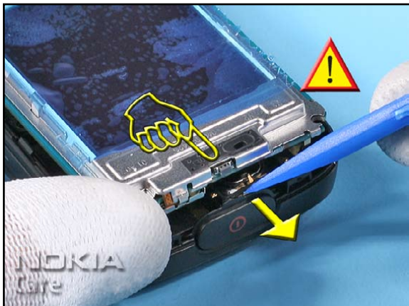
12. First, bend back the power key a bit to avoid damaging of the power switch and then place the ENGINE MODULE onto the B-COVER.
