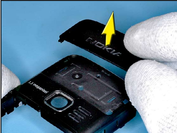
37. Remove the TOP COVER from the B-COVER.
