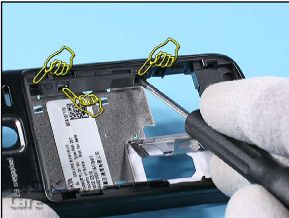
27. Turn the B-COVER and release the three snaps in front of SIM door.
