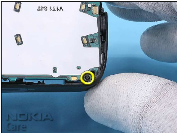
9. Gently, remove the ENGINE MODULE. Avoid damaging the guide pin of the B-COVER.
