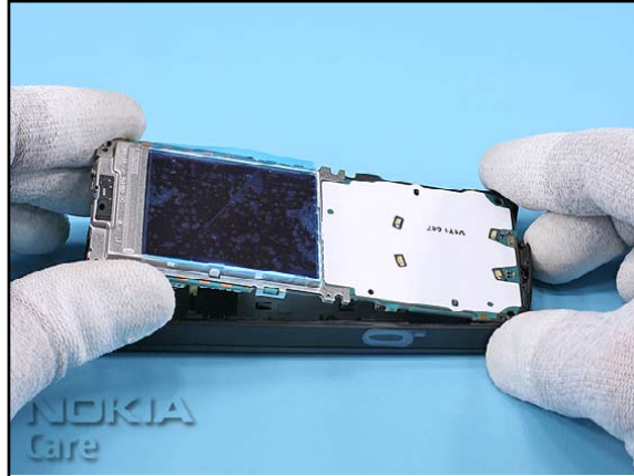
8. Lift the Engine Module a bit as shown.
