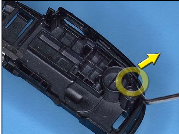
38. Release the snap from the CONNECTOR in the edge with the dental tool.
